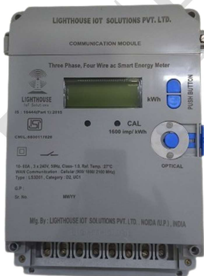
Three Phase Smart Energy Meter
